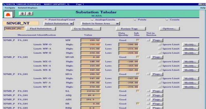
Fig. 2. Substation Tabular Presentation
